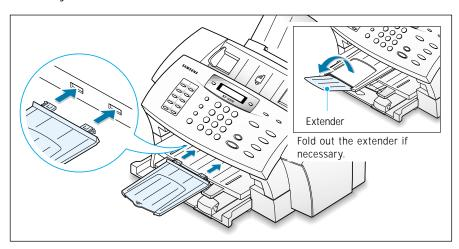
Note: The SF-4700 is shipped with the paper output tray already installed. Extend the tray to use.
